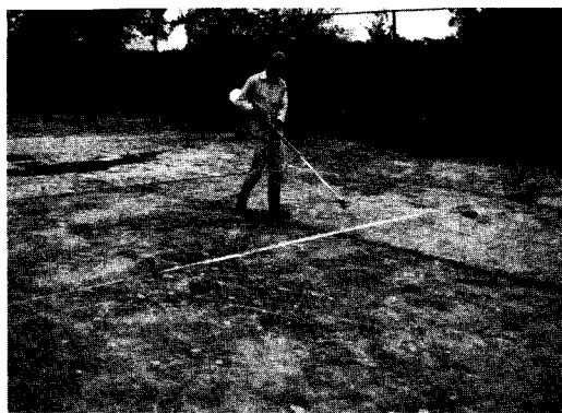
Plate 2. Single pass made at the centre of the water-sensitive paper for monitoring the spray distribution and droplet density.
