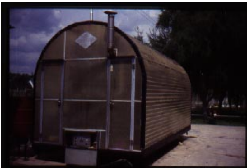
Gambar 2. Mesin pengering saiz komersial menggunakan tenaga suria dan diesel (Commercial sized dryer with solar and diesel energy)
