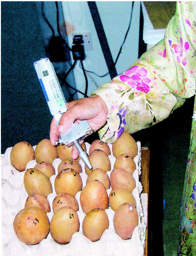
Plate 1. Sapodilla fruits placed on the fibreboard tray for firmness measurement using the Kiwifirm device
