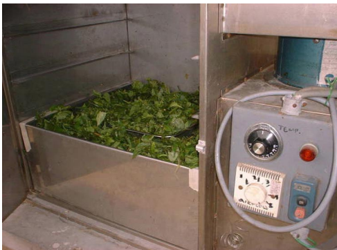
Plate 1. Drying of kenaf using small dryer in laboratory
