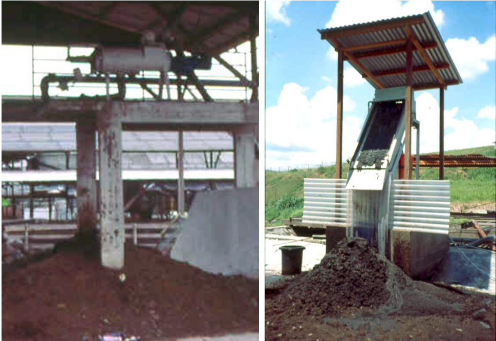
Plate 1. Screw-press separator (left) and inclined screen separator (right)
