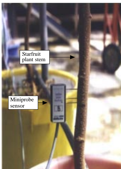
Plate 1. Miniprobe sensor inserted into stem of starfruit plant
