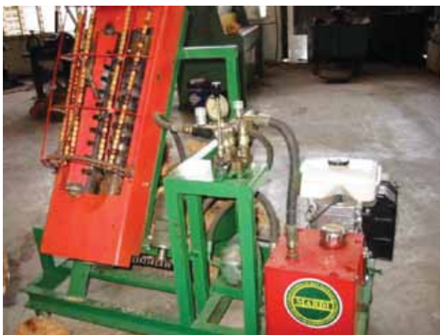
Plate 1. Major components of the coconut dehusking machine
