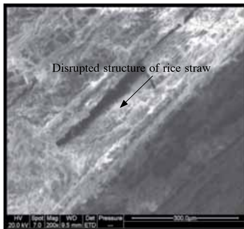
Figure 4b. Surface of rice straw treated with bacteria under X500 magnification using scanning electron microscope
