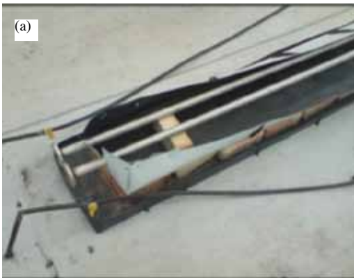
Plate 3. (a) Two rows of 25 mm diameter stainless steel pipe used in root zone cooling. (b) Pipe network and solenoid valves installed for root zone cooling
