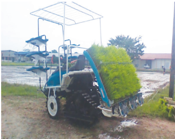
Figure 3. Paddy transplanter with triangular steel track system
