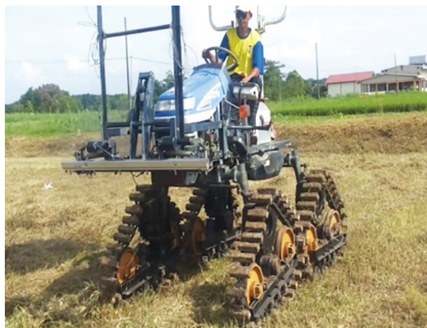
Figure 2. High clearance prime mover with triangular track system using wooden shoes
