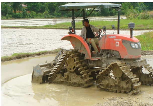
Figure 1. Tractor equipped with four half tracks
