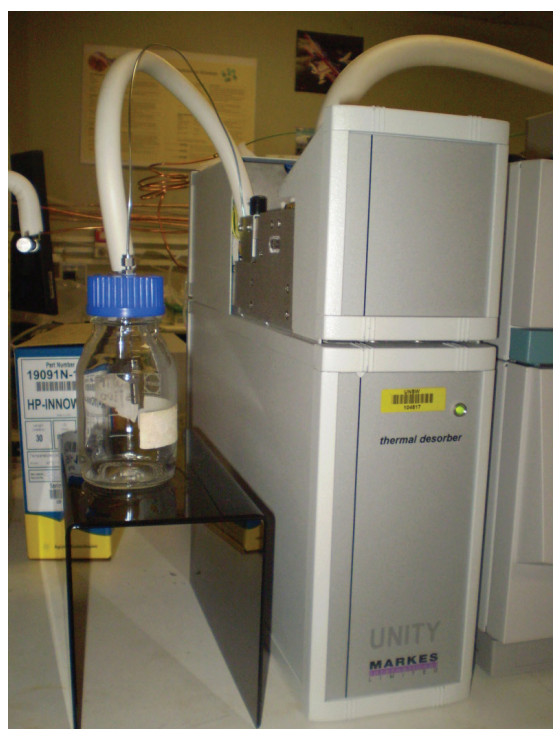
Figure 1. Direct headspace sampler showing sample vessel and thermal desorption unit (Markes International, UK)
