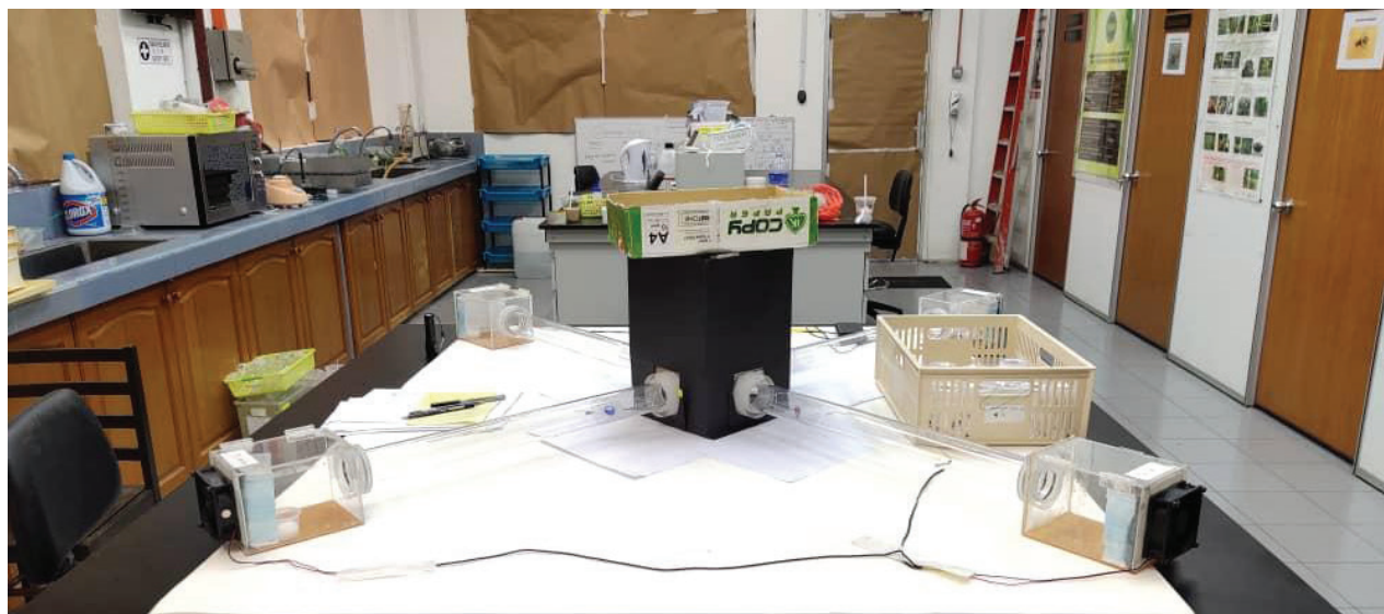
Image 2. Experimental arena for choice assay using a four-arm olfactometer
